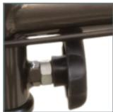
Insert the Steering Safety Lock ⑧ below the frame on the steering column. Tighten the knob firmly till none of the threads are showing. This is to prevent the axle from over-rotating. Failure to do so may result in tipping or an abrupt stop causing serious injury. Axle/handlebar movement should be no more than approximately 45 degrees left and right.
