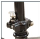
The quick release clamp ③ at the base of the steering column should now be facing forward. The clamp has an added security pin to prevent it from collapsing during use. Release the lever and swing it down and away from the steering column. Push
